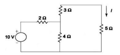
b) Determine the Maximum Power Delivered to the load in the circuit shown
