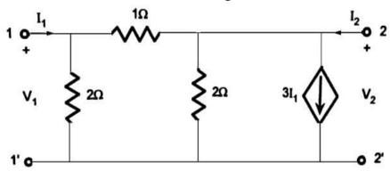
b) Determine the Open Circuit Parameters from the given Circuit shown.
